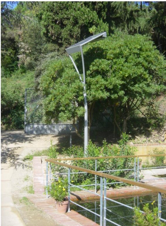
The photovoltaic solar module uses a 0,9 sq. m. receptor panel fixed to an inclined structure at the apex of the streetlight. It generates 135 Wp of power.
